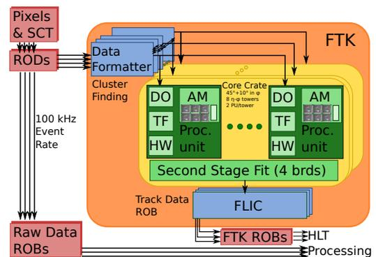
Fig. 1. Architecture of FTK system. AM is the Associative Memory, DO is the Data Organizer, FLIC is the FTK-to-Level-2 Interface Crate, HW is the Hit Warrior, ROB is the ATLAS Read Out input Buffer, ROD is a silicon detector Read Out Driver, and TF is the Track Fitter. Second Stage Fit is referred to in the text as the Second Stage Board.
