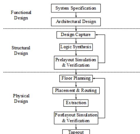
Fig. 1. Digital design flow steps
