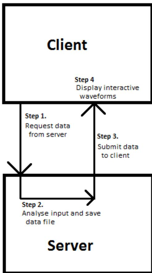
Fig. 1. The client requests data from the server which analyzes the input (VCD file) and returns them in an easy to process format.
