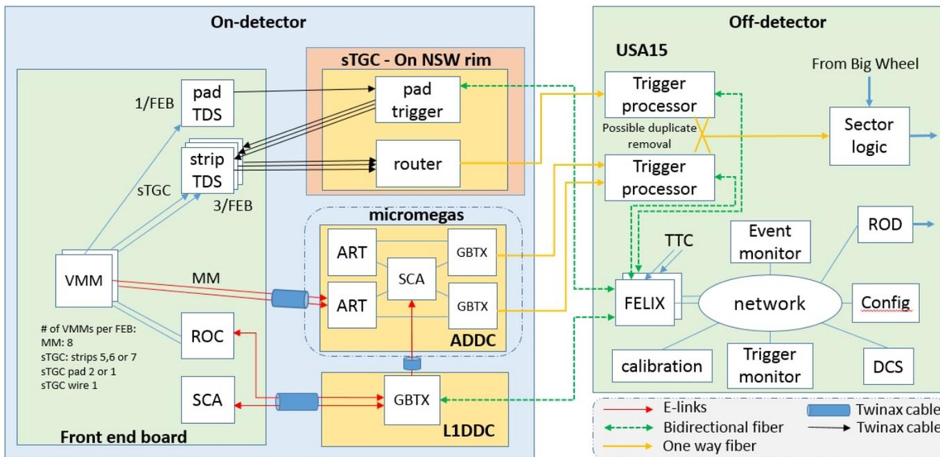
Fig. 1: NSW electronics trigger and dataflow. L1DDC is connected to the ROC and the SCA ASIC of the front-end boards with one e-link each. One e-link and two extra differential pairs are used for the connection to the ADDC boards and a bidirectional optical link is used for the communication to the FELIX.
