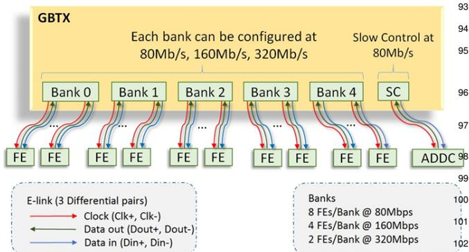
Fig. 3: GBTX e-link connectivity. There are five banks which support up to 40 FE boards. In each bank eight FE boards can be connected at 80 Mbps, four at 160 Mbps or two at 320 Mbps. An extra Slow Control e-link with a fixed rate at 80 Mbps is used for the connection to the ADDC board.
