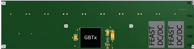
163 (b) Bottom side. The GBTX ASIC, the DC-DC converters and the position pins
