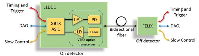
Fig. 2: On the left side the L1DDC, which resides on the detector and is implemented with custom ASICs, combines the three distinct paths (Timing and Trigger, DAQ, Slow Control) into a single bidirectional optical link.
