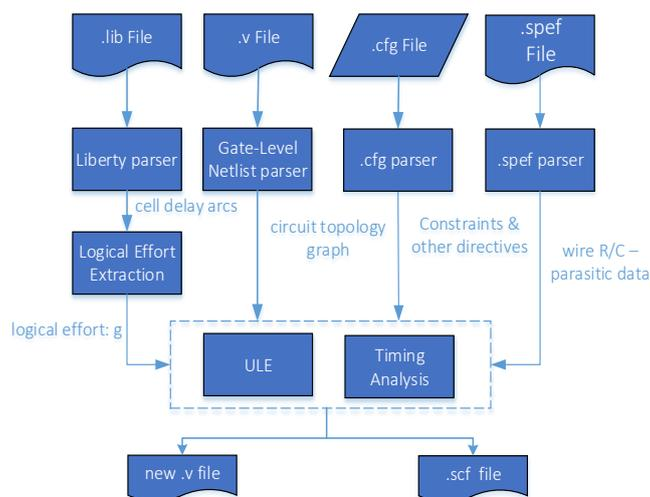
Figure 1 - Software Architecture
