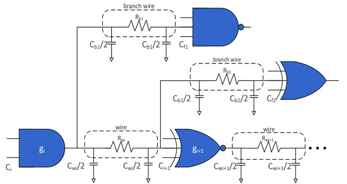
Figure 2 A logic path segment including RC interconnect and two branches
