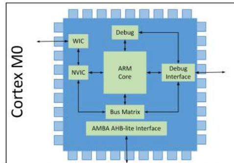
Fig. 2. Inner Architecture of  $\mu\text{C}$
