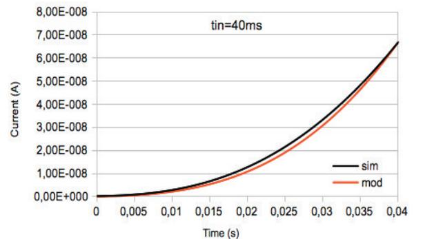
Fig. 2. Comparison between the model predictions and simulations of a OTFT transistor for the fastest input rise time  $t_{in}$ .
