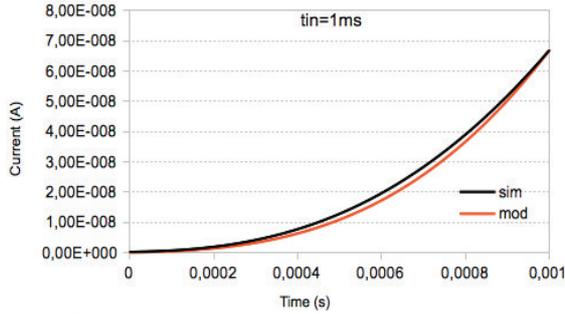
Fig. 3. Comparison between the model predictions and simulations of a OTFT transistor for the slowest input rise time  $t_{in}$ .
