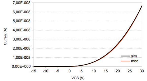
Fig. 1. Comparison between the nth-power law model predictions and simulations for a OTFT transistor.
