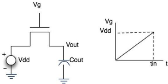
Fig. 4. Circuit under delay analysis. Initially,  $V_{out}=0$ .
