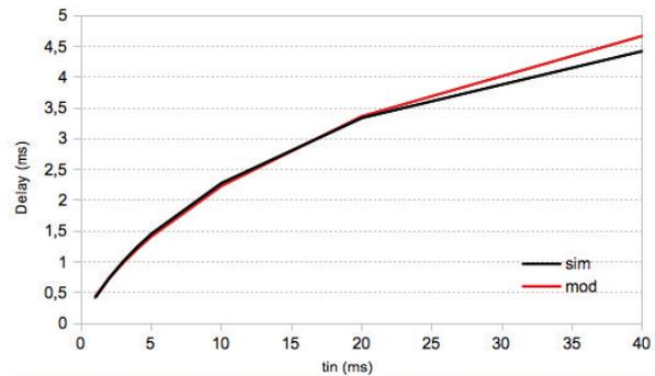
Fig. 5. Comparison between simulated (black) and modelled (red) delay times for a 1pF load.
