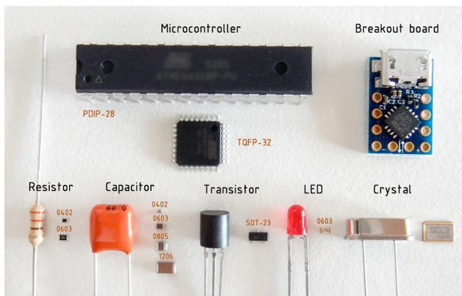
Fig. 1. Surface-mount vs through-hole components and breakout boards
