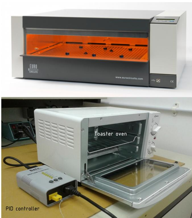
Fig. 5. Commercial (top) and converted reflow ovens (bottom)
