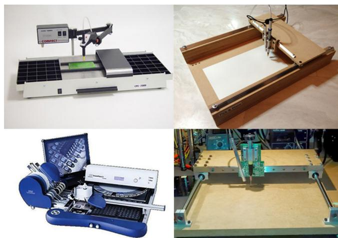
Fig. 4. Commercial (left) and custom (right) manual pick-and-place devices
