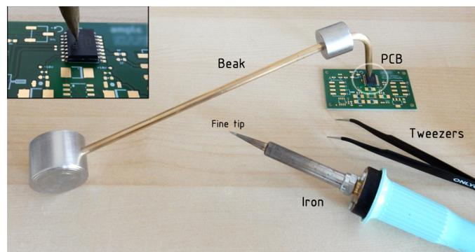
Fig. 2. SMD hand-soldering tools
