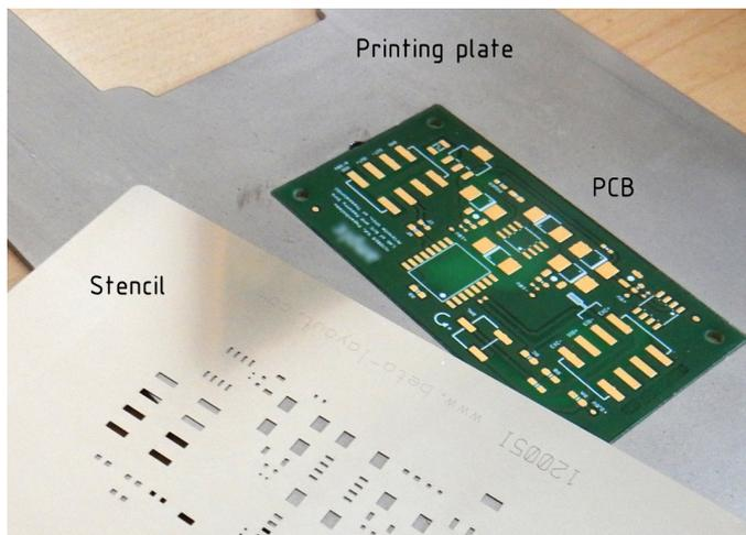
Fig. 3. Manual solder paste printing
