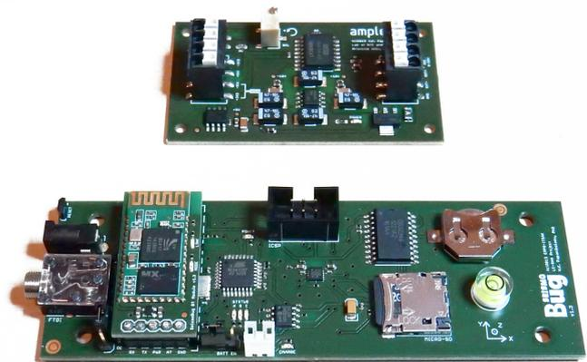
Fig. 6. Miniature strain gauge amplifier (top), autonomous triaxial accelerograph (bottom).
