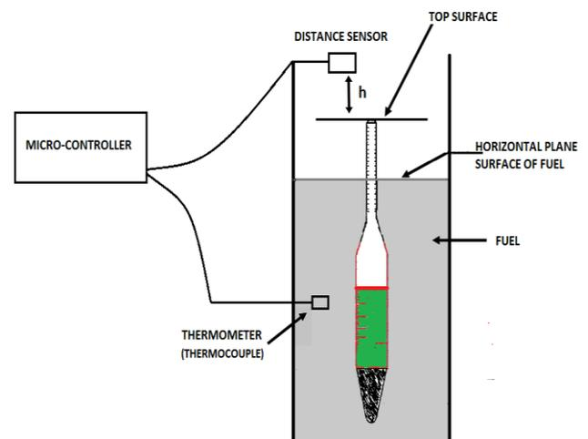
Fig. 1. The sensing device
