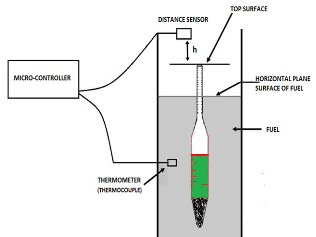
Fig. 1. The sensing device
