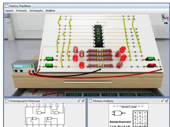
Fig. 4. The Web-based digital circuit Virtual Lab
